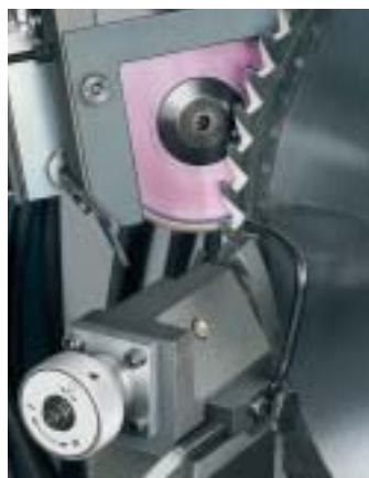
Grinding of roughing and finishing tooth chamfers on HSS saw blades
