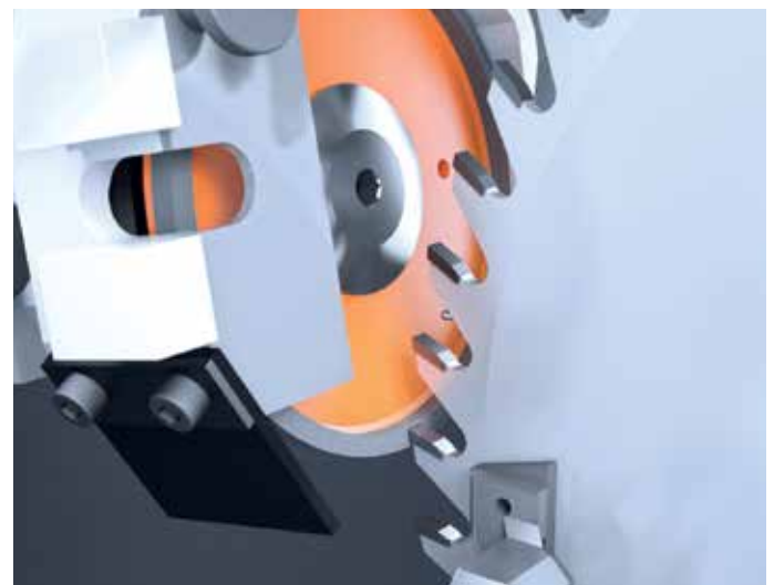
/// TOOTH TOP MACHINING
